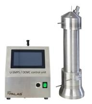
A soft X-ray source as a neutralizer is already integrated. The advantage instead of a radioactive neutralization (for example, with Kr-85) is that there is no need to follow requirements during transportation.
