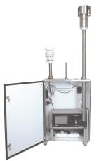
The Fidas® 200 S version is a 19" plug-in unit mounted in a splash-proof stainless steel control cabinet for outdoor use (temperature range -20 - 50 °C). A larger, air-conditioned control cabinet is available on request, allowing the installation of additional devices. Variants of the Fidas® 200 S are the basic Fidas® 200 and the Fidas® 200 E with a remote sensor (for easier integration into stations with existing roof feed-through).
