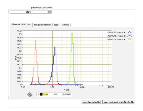
Display of all measured single particles and the corresponding statistics for distributions in table form
