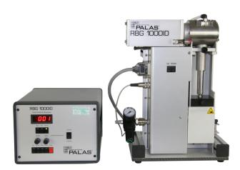
The dispersion unit and the electrical control unit can be set up up to  $2\,\mathrm{m}$  apart from each other.
