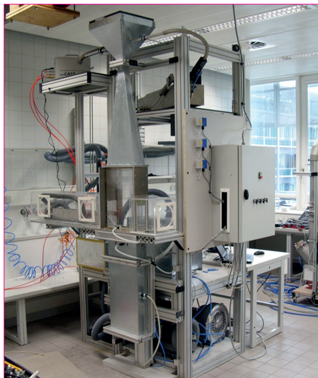
Fig. 7: Drum filter test bench at the Institute of Process Engineering, Environmental Technology and Technical Biosciences of the Vienna University of Technology
