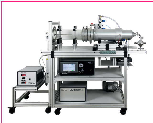
Fig. 5a) Test bench MMTC 200 for cleanable filter media, horizontal raw gas conduit (Image: Palas GmbH)
