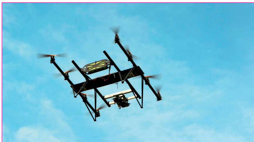
Fig. 4: Octocopter HORUS with a Fidas Ultra-Light Sensor (Image: Palas GmbH)
