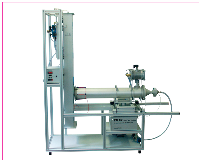
Fig. 5b) Test bench MMTC 3000 for cleanable filter media, vertical raw gas conduit (Image: Palas GmbH)
