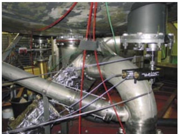
welas ® sensor under the AIDA aerosol chamber: the chamber is located within a coolable housing. A sample from the aerosol chamber is taken out continuously through the vertically running stainless steel tube.
