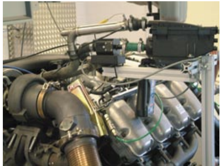
Engine test rig for the characterisation of oil separators at Donaldson Coordination Center B.V.B.A. in Belgian Leuven
