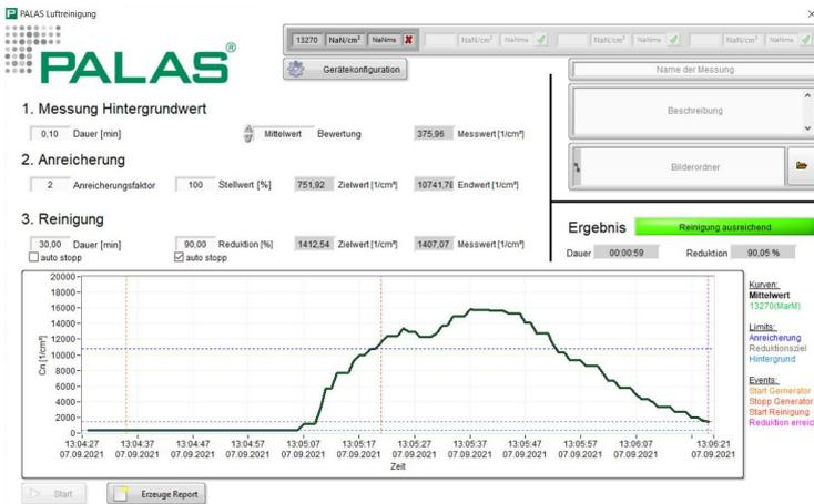
With the AQControl software, in addition to indoor air quality, effectiveness tests for room air cleaners can be carried out directly on-site (real room situation) - even if no person is present.
