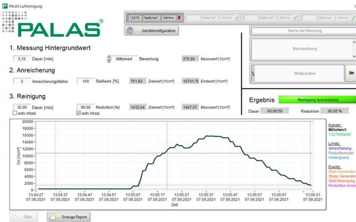
With the AQControl software, in addition to indoor air quality, effectiveness tests for room air cleaners can be carried out directly on-site (real room situation) - even if no person is present.
