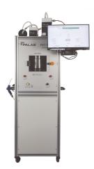
The FET 100 enables testing of the smallest filter elements up to  $100 \times 100$  mm, such as medical filters, vacuum cleaner end filters, and fan filters. Coarse filters up to ULPA filters are tested for particle size separation and differential pressure. The FET 100 measures better than required by the standards. Thanks to individual adapters and customer-specific adjustments in the air duct, the FET system can be used for a wide variety of filter elements.
