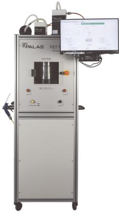
The FET 100 enables testing of the smallest filter elements up to 100 x 100 mm, such as medical filters, vacuum cleaner end filters, and fan filters. Coarse filters up to ULPA filters are tested for particle size separation and differential pressure. The FET 100 measures better than required by the standards. Thanks to individual adapters and customer-specific adjustments in the air duct, the FET system can be used for a wide variety of filter elements.
