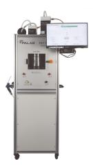
To reliably determine the quality and efficiency of filter elements, it is crucial to test energy consumption (pressure drop), loading, particle separation efficiency, and total penetration.
