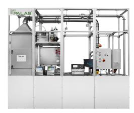
The FET 600 enables defined testing of filter elements up to 610 • 610 mm, such as ventilation filters, HEPA/ULPA filters, vacuum cleaner filters, and car cabin filters. Designed for optimum flow guidance, the channel can also use adapters for smaller filter elements. Coarse filters up to ULPA filters are tested for separation via particle size and differential pressure.
