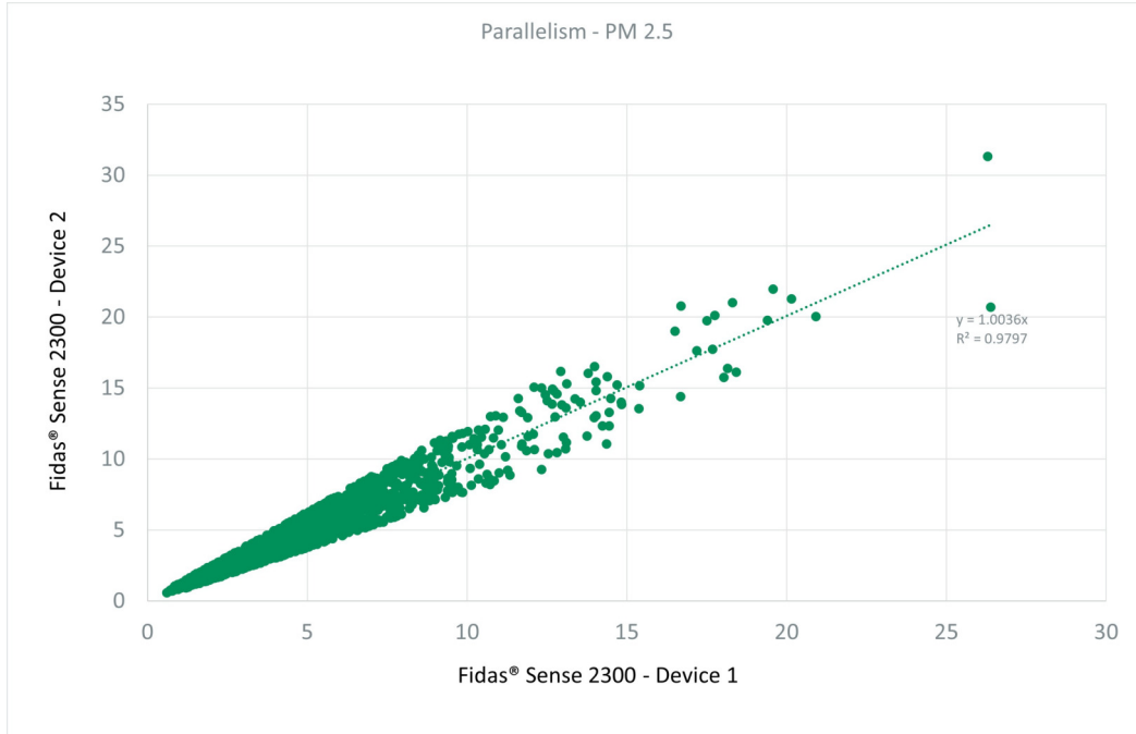
Pic.1: Parallelism of two Fidas® Sense 2300 systems
