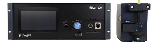
The new P-DAP 2000 system for emission measurement is equipped with a highly resolving aerosol photometer for an extensive measurement range of mass concentration which is specially developed for the operation in monitoring applications.
