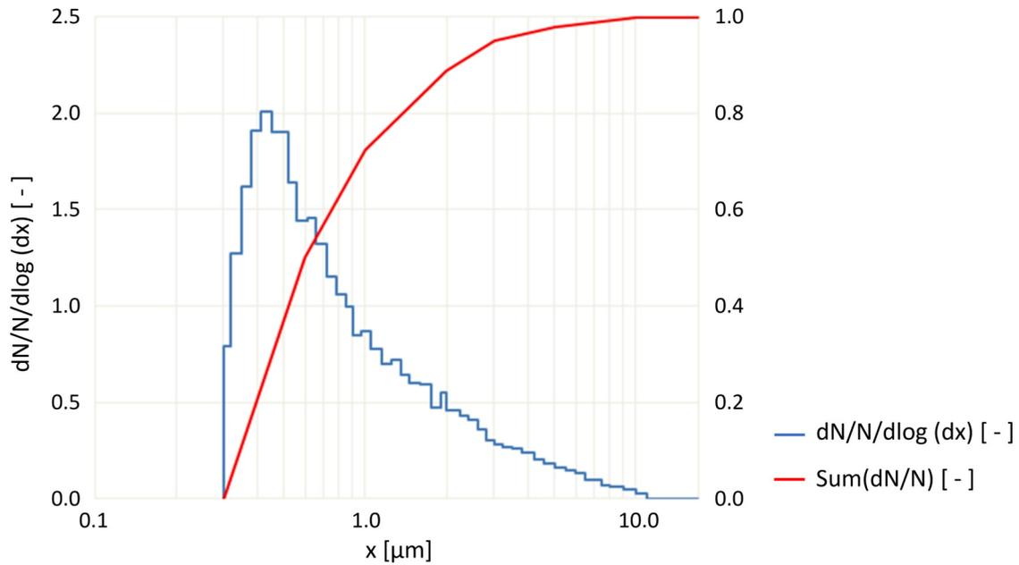
Fig. 2: Particle size distribution with the welas<sup>®</sup> digital 2000
