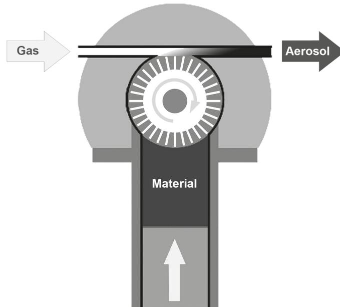
Fig. 1: Schematic diagram of RBG system
