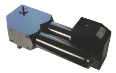
The model 1100 aerosol sensors are equipped with a small measurement volume and are used for coincidence-free measurement with a max. number concentrations up to 500,000 particles/cm<sup>3</sup>. Measuring range:  $0.12 - 3.5 \, \mu \text{m} / 0.2 - 10 \, \mu \text{m} / 0.3 - 17 \, \mu \text{m} / 0.6 - 40 \, \mu \text{m}$ .
