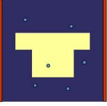
For concentrations up to 500,000 particles/cm<sup>3</sup>, the welas<sup>®</sup> 1100 sensor with a very small measuring volume is used. This ensures the smallest measuring volume such that only one particle ever enters the measuring volume. In low concentrations, the model welas<sup>®</sup> 1200 with a larger measuring volume offers the advantage of a higher counting rate at the same number concentration.
