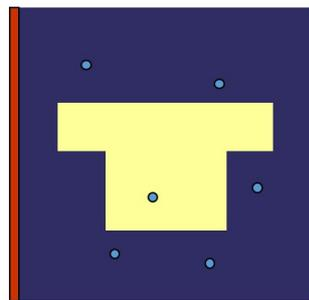
For concentrations up to 500,000 particles/cm<sup>3</sup>, the welas<sup>®</sup> 1100 sensor with a very small measuring volume is used. This ensures the smallest measuring volume such that only one particle ever enters the measuring volume. In low concentrations, the model welas<sup>®</sup> 1200 with a larger measuring volume offers the advantage of a higher counting rate at the same number concentration.
