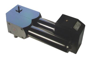
The model 1200 aerosol sensors are equipped with a small measurement volume and are used for coincidence-free measurement with a maximum number of concentrations of up to 50,000 particles/cm $^3$ . Measuring range: 0.12 – 3.5  $\mu$ m / 0.2 – 10  $\mu$ m / 0.3 – 17  $\mu$ m / 0.6 – 40  $\mu$ m.
