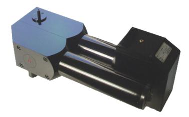
The model 1200 aerosol sensors are equipped with a small measurement volume and are used for coincidence-free measurement with a maximum number of concentrations of up to 50,000 particles/cm<sup>3</sup>. Measuring range:  $0.12-3.5~\mu\text{m}/0.2-10~\mu\text{m}/0.3-17~\mu\text{m}/0.6-40~\mu\text{m}$ .
