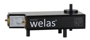
The model 2070 aerosol sensors are equipped with a very small measurement volume and are used for coincidence-free measurement with a maximum number of concentrations up to 1,000,000 particles/cm³ and in the highest mass concentrations, e.g., Arizona dust A2, SAE Fine, up to 1,000 mg/m³. Measuring range: 0.2 – 10  $\mu$ m / 0.3 – 17  $\mu$ m / 0.6 – 40  $\mu$ m.
