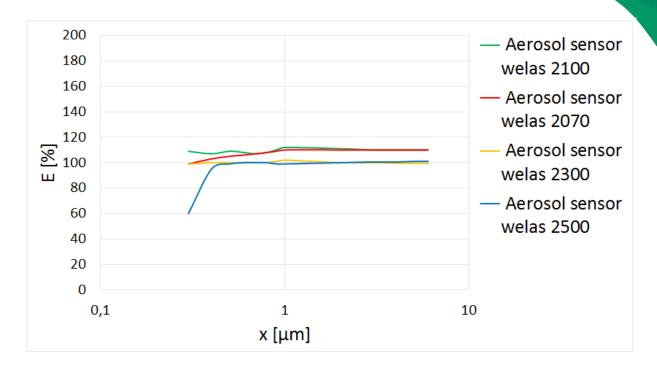
Graph 1: Counting efficiency of various sensors in relation to the welas<sup>®</sup> 2200 sensor (in the measuring range 0.2 –  $10 \mu m$ )
