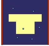
For concentrations up to 1,000,000 particles/cm<sup>3</sup>, the welas<sup>®</sup> 2070 sensor with a small measuring volume is used. This ensures the smallest measuring volume such that only one particle ever enters the measuring volume. In low concentrations, the models with a larger measuring volume offer a higher counting rate at the same number concentration.
