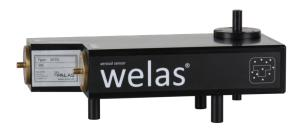
The model 2070 aerosol sensors are equipped with a very small measurement volume and are used for coincidence-free measurement with a maximum number of concentrations up to 1,000,000 particles/cm³ and in the highest mass concentrations, e.g., Arizona dust A2, SAE Fine, up to 1,000 mg/m³. Measuring range: 0.2-10  $\mu$ m / 0.3-17  $\mu$ m / 0.6-40  $\mu$ m.
