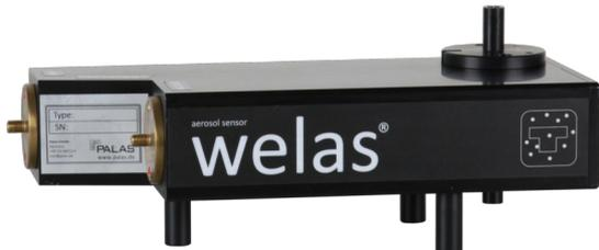
The model 2100 aerosol sensors are equipped with a small measurement volume and are used for coincidence-free measurement with a maximum number concentrations of up to 500,000 particles/cm<sup>3</sup>. Measuring range: 0.2 – 10  $\mu\text{m}$  / 0.3 – 17  $\mu\text{m}$  / 0.6 – 40  $\mu\text{m}$ .
