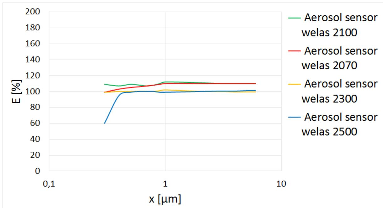
Graph 1: Counting efficiency of various sensors in relation to the welas<sup>®</sup> 2200 sensor (in the measuring range 0.2 – 10 µm)
