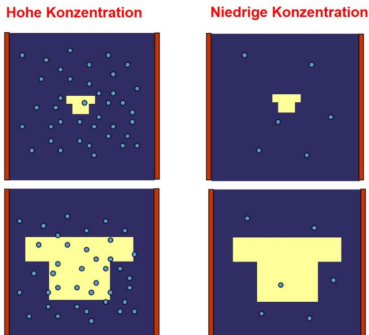
For concentrations up to 1,000,000 particles/cm<sup>3</sup>, the welas<sup>®</sup> 2070 sensor with a small measuring volume is used. This ensures the smallest measuring volume such that only one particle ever enters the measuring volume. In low concentrations, the models with a larger measuring volume offer a higher counting rate at the same number concentration.
