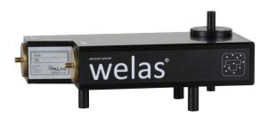
The model 2500 aerosol sensors are equipped with a very big measurement volume and are used for coincidence-free measurement with a maximum number concentrations up to 4,000 particles/cm³. This aerosol sensor allows statistically reliable measurements in low raw gas concentrations down to clean room class 100,000 and for filter testing according to ASHRAE 52.2. Measuring range:  $0.3-17~\mu m$  /  $0.6-40~\mu m$  /  $2-105~\mu m$ .
