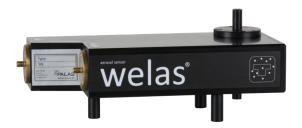
The model 2500 aerosol sensors are equipped with a very big measurement volume and are used for coincidence-free measurement with a maximum number concentrations up to 4,000 particles/cm<sup>3</sup>. This aerosol sensor allows statistically reliable measurements in low raw gas concentrations down to clean room class 100,000 and for filter testing according to ASHRAE 52.2. Measuring range:  $0.3-17~\mu m / 0.6-40~\mu m / 2-105~\mu m$ .
