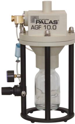
The AGF 10.0 is an aerosol generator for atomizing liquids and latex suspensions with a constant particle rate and defined particle spectrum.
