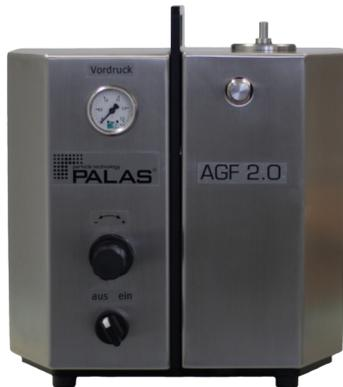
The AGF 2.0 is an aerosol generator for atomizing liquids and latex suspensions with a constant particle rate and defined particle spectrum.
