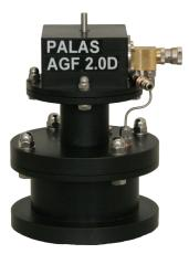
Unlike the AGF 2.0, the AGF 2.0 D is pressure-resistant up to 10 bar positive pressure and is thus able to be used for applications with an absolute pressure value of up to 11 bar, e.g., to test compressed air filters and optical flow measurement procedures with positive pressure values of up to 10 bar.
