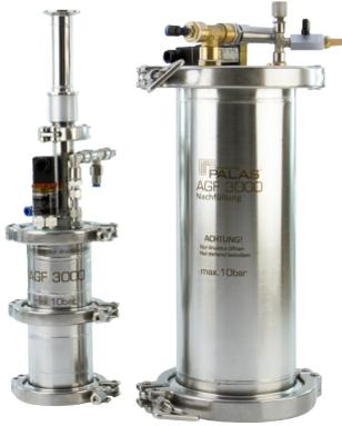
The AGF 3000 was specially developed to supply compressed air filters per ISO 12500 until the compressed air filter is saturated. The AGF 3000 system comprises an aerosol generator and an automatic refill unit.
