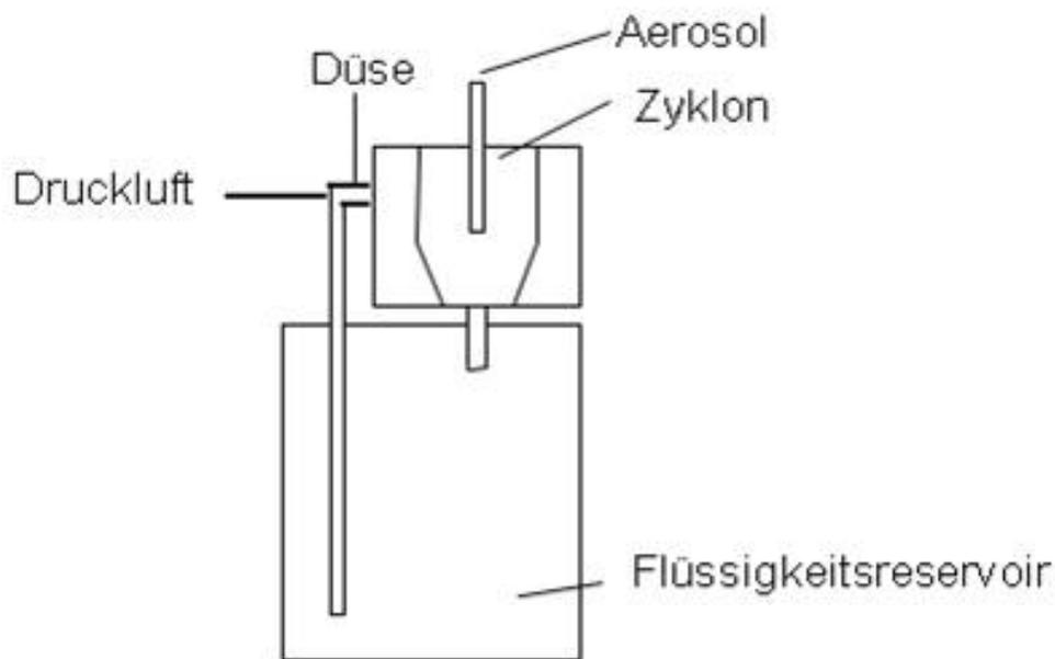
Fig. 1: Schematic diagram of the AGK 2000 with cyclone
