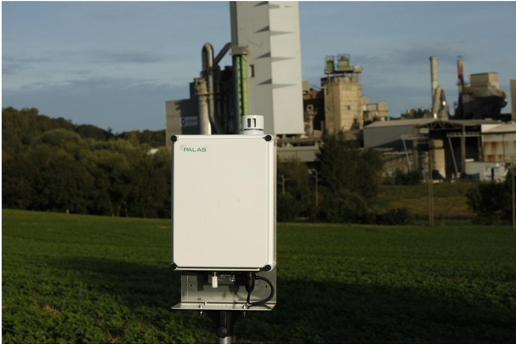
Fig. 1: AQ Guard Smart on a tripod
