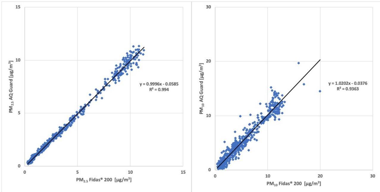
Fig. 2: Comparison of data recorded by AQ Guard and Fidas<sup>®</sup> 200 S
