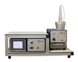
The BEG 2000 is equipped with automatic mass flow control. For this purpose, the dosing unit of the BEG 2000 is continuously weighed. The data is constantly recorded and evaluated by a touchscreen PC via a serial interface.
