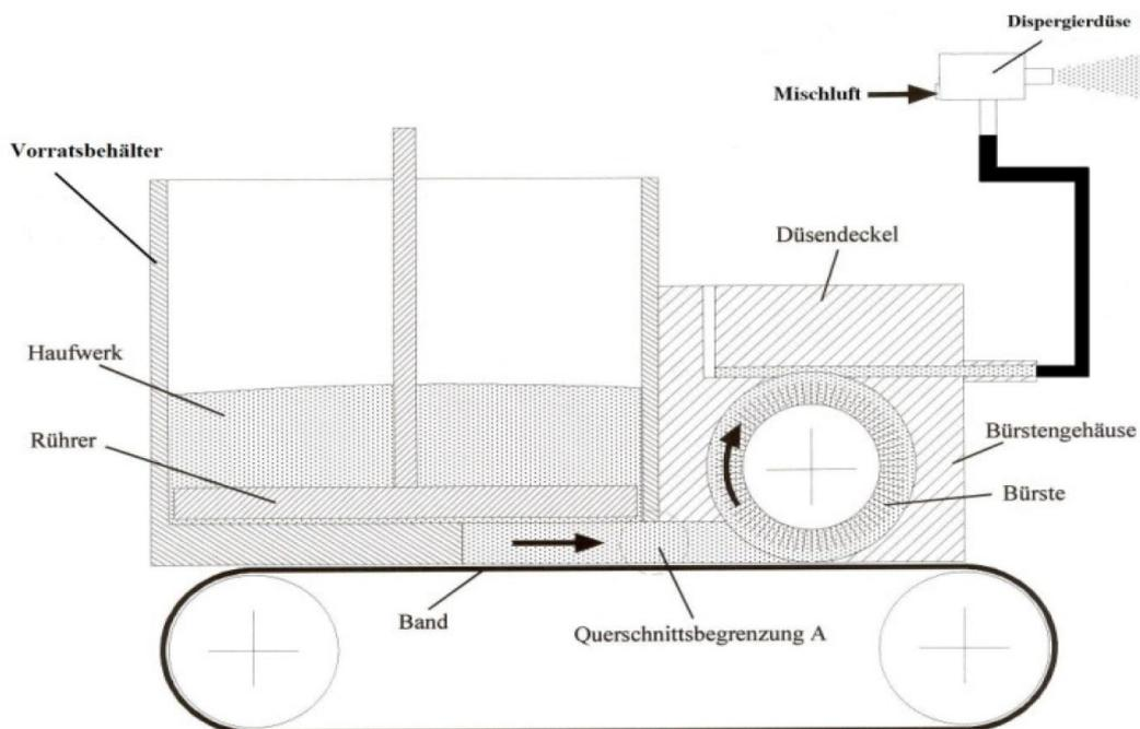
Fig. 1: Principle of operation of the BEG 1000/BEG 2000
