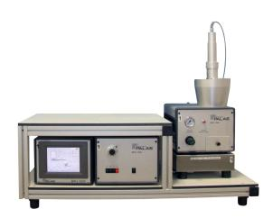
This dispersion system can continuously generate low mass flows, e.g.,  $8\,g/h$ , with optimal dosing constancy and control with automatic mass flow monitoring. Mass flow setting of approx. 8 g/h – 550 g/h based on SAE fine, A2 dust.
