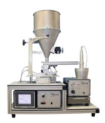
This dispersion system can continuously generate low mass flows, e.g.,  $8\,g/h$ , with optimal dosing constancy and control with automatic mass flow monitoring. The automatic refill and weighing units enable this dispersion system to be successfully used for continuous dosing over several days. Mass flow setting of approx.  $8\,g/h - 550\,g/h$  based on SAE fine, A2 dust.
