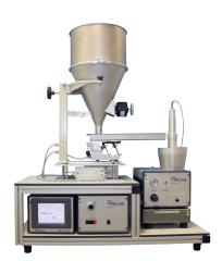
This dispersion system can continuously generate low mass flows, e.g.,  $8\,g/h$ , with optimal dosing constancy and control with automatic mass flow monitoring. The automatic refill and weighing units enable this dispersion system to be successfully used for continuous dosing over several days. Mass flow setting of approx.  $100\,g/h - 6\,kg/h$  based on SAE fine, A2 dust
