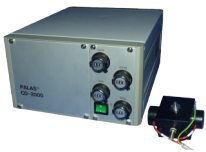
CD 2000 Type A Bipolar discharge unit with lower mixed air flow
