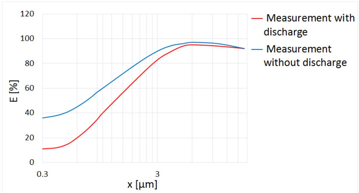
Fig. 2: Fractional separation efficiency with and without CD 2000
