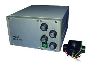
The CD 2000 type B bipolar discharge unit uses a mixed airflow of  $3-36\ m^3/h$  with a tube diameter on the aerosol inlet of  $\emptyset$ i= 13 mm.
