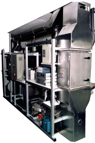
For standard tests on automotive cabin air filters according to DIN 71460-1 and ISO/TS 11155-1, Palas offers the CIF 1000 test stand with the **Promo® 1000<sup>1</sup>**.
