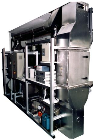
Palas offers the CIF 3000 test rig with the **Promo® 3000**<sup>1</sup> unit for standard tests on motor vehicle passenger compartment filters in accordance with DIN 71460-1 and ISO/TS 11155-1.
