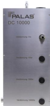
The DC 10000 consists of four cascaded special dilution systems with a dilution factor of 1:10. The DC 10000 dilution cascade has one aerosol inlet and four aerosol outlets. Depending on which aerosol outlet is connected to the measuring device, the aerosol with the dilution factors 1:10, 1:100, 1:1,000, or 1:10,000 are diluted.
