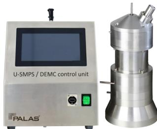
The DEMC size classifier (as defined in ISO 15900:2000) selects aerosol particles from an aerosol stream according to their electrical mobility. Different lengths of columns are available depending on the size range to be selected. Depending on the configuration of the control unit and column, the designation changes accordingly.
