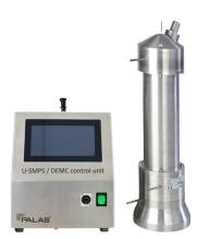
A soft X-ray source as a neutralizer is already integrated. The advantage instead of a radioactive neutralization (for example, with Kr-85) is that there is no need to follow requirements during transportation.
