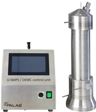
A soft X-ray source as a neutralizer is already integrated. The advantage instead of a radioactive neutralization (for example, with Kr-85) is that there is no need to follow requirements during transportation.
