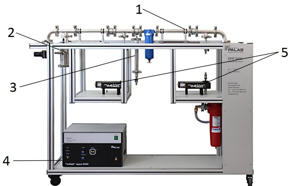
1. Mobile test set-up, easy filter changes thanks to the movable clean gas section: Thanks to the movable clean gas section, filter housings of different sizes can be used without difficulty
