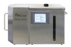
The DLB 2000, well established in practice, ensures fully automated regulation of rel. humidity with maximum stability. The input of the required rel. humidity and setting of the temperature take place using a touchscreen display.
