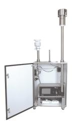
The Fidas<sup>®</sup> 200 S version is a 19" plug-in unit mounted in a splash-proof stainless steel control cabinet for outdoor use (temperature range -20 - 50 °C). A larger, air-conditioned control cabinet is available on request, allowing the installation of additional devices. Variants of the Fidas<sup>®</sup> 200 S are the basic Fidas<sup>®</sup> 200 and the Fidas<sup>®</sup> 200 E with a remote sensor (for easier integration into stations with existing roof feed-through).
