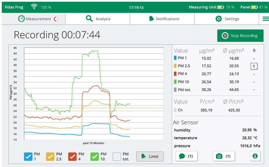
Fig. 3: Display of measured values during a measurement
