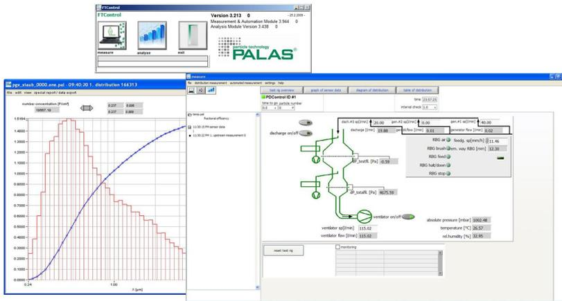
The FTControl software is used for the reliable and economic performance of filter tests and fractional separation efficiency measurements with the welas<sup>®</sup> digital and Promo<sup>®</sup> optical aerosol spectrometer.
