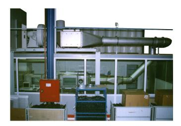
Upgrading and automation of particle measurement with the GVT 3000 (General Ventilation Test System Upgrade), serves in quality assurance and the development of filters in EN 779, ASHRAE 52.2, and ISO 16980 test rigs. The upgrade consists of an aerosol spectrometer, incl. a laptop/PC and monitor, aerosol generators (optionally: discharge unit), a sampling system, as well as automation of the measurement process.
