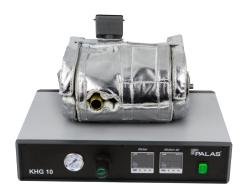
The KHG 10 series of heatable dilution systems builds upon the VKL series ejector principle. In addition to the advantages of the VKL series, the KHG series dilution system is configured to be heatable to  $150\,^{\circ}$ C (optionally up to  $200\,^{\circ}$ C) and is additionally pressure-resistant up to  $10\,^{\circ}$ bar pressure. Isothermal and isobaric dilution can therefore be achieved. With the KHG system, both the compressed air supplied and the dilution system are self-heated.
