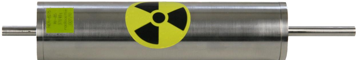
The Kr-85 Neutralizer is a bipolar neutralizer that generates positive and negative ions through ionization with the emitted  $\beta$  radiation. Suppose these ions are brought together with an aerosol; a defined equilibrium charge distribution is established, as is necessary for measuring systems, such as scanning mobility particle sizers (e.g., Palas U-SMPS system). This neutralizer is available in two versions with different activities, 75 MBq, and 370 MBq.
