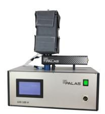
The dilution of large droplets is significant when measuring highly concentrated droplet aerosols. Since large droplets are challenging to dilute, standard systems only work up to a size of 1 - 2  $\mu$ m. The model variant LDD 100 H can be heated up to  $150\,^{\circ}\text{C}$  and thus prevents condensation.
