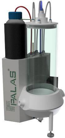
With the conversion of the test standards for the general room air filters from EN 779 to ISO 16890, an additional test aerosol (KCl) with particle sizes of up to 10  $\mu\text{m}$  is required, which remains stable even at low flow rates. Palas is the first manufacturer to produce such an aerosol to test filter media. The LSPG 16890 enables stable and reproducible atomization of NaCl and other salt solutions.
