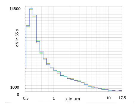
Fig. 1: Reproducible particle size distribution from KCl up to 10  $\mu m$  in the MFP 3000
