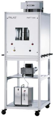
The MFP filter test rig is a modular filter testing system for flat filter media and small filters. The MFP 1000 can be used to determine pressure loss curve on the medium without a dust coating, fraction separation efficiency, or burden and fraction separation efficiency during application of the burden within shortest times – reliably and therefore cost-effectively.
